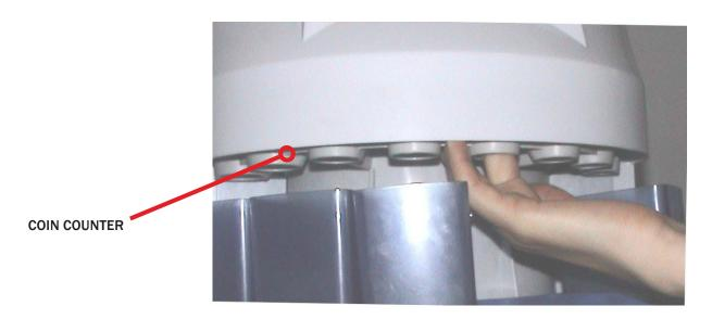
If the machine isn't put on the horizontal or it shakes too much when it's working, sometimes a coin will falls in a smaller Coin Channel by error and then it will cause a jam.
